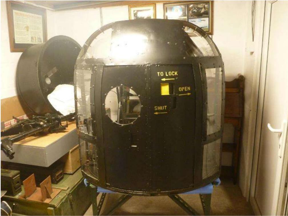
Seen below is the drum and floor assembly with the rotating turret ring in the spray shelter. I took a gamble on fitting the turret ring before spraying as I'm pretty certain that the two fixed turret rings can be fitted to this complete assembly.
